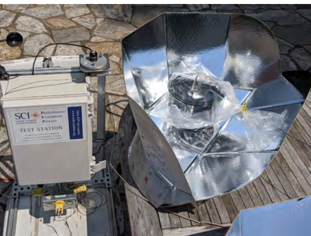
▲ Test station with CookKit reflective panel solar cooker with oven bag. Photo by SCI.
