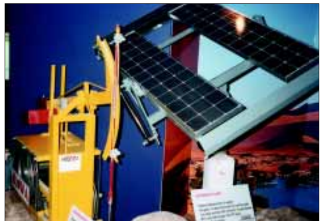
Wind-power model (left), and PV-driven deep-well pump (right) from Namibia
