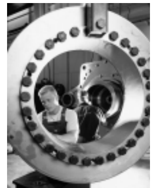
Assembly wind mill hub. Photo by NEG MICON.
