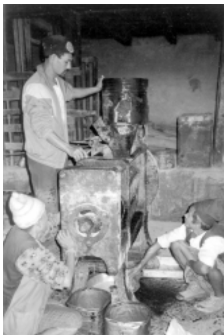
Extracting mustard from seeds in Nepal. The mill runs by a micro-hydro plant. Photo by REDP.
