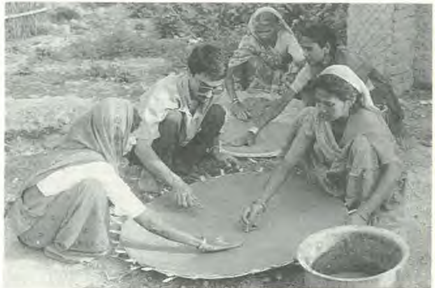
Solar cooker under construction by women from untouchable caste in Nepal.
