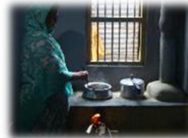
Improved cookstove (single Burner, with chimney)
