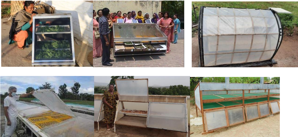
Séchoirs solaires dryers: Cabinet model from wood and glas (CRT, Nepal), cabinet from metal and glas (AIWC, India), Poly-Tunnel model from Bamboo, (INSEDA, India), and semi-industrial models (PHilMech) in the Philippines, and ESFRITA & TaTEDO in Tanzania.
