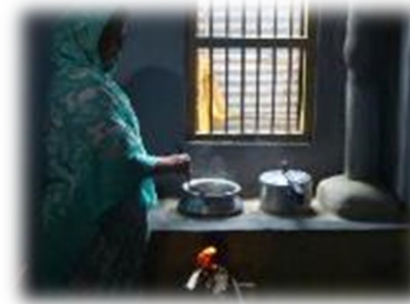
Improved cookstove (single Burner, with chimney)
