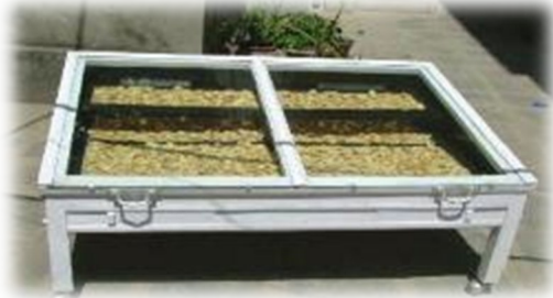
Cabinet Solar Dryer
