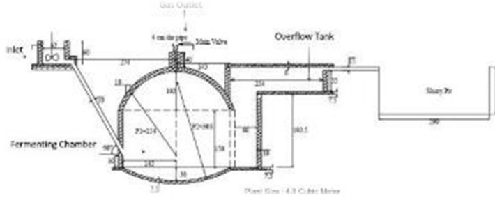
Household Biogas Plant
