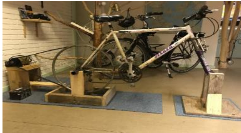
Static bike for charging power banks
