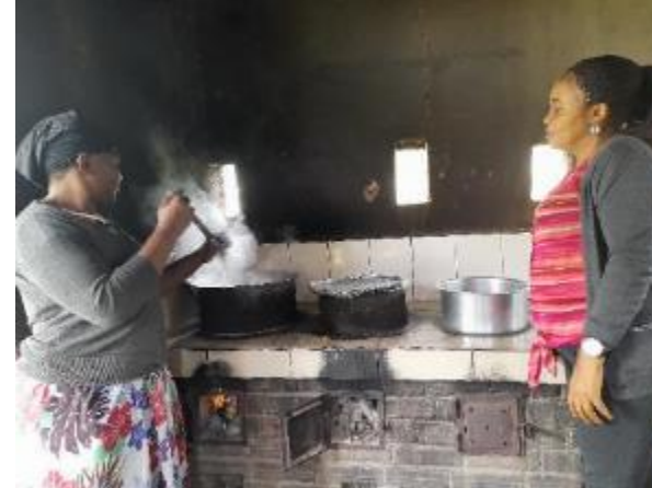
Replacement of inefficient with efficient stove reduce amount of fuelwood consumption by more than half
