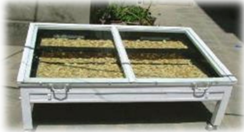
Cabinet Solar Dryer
