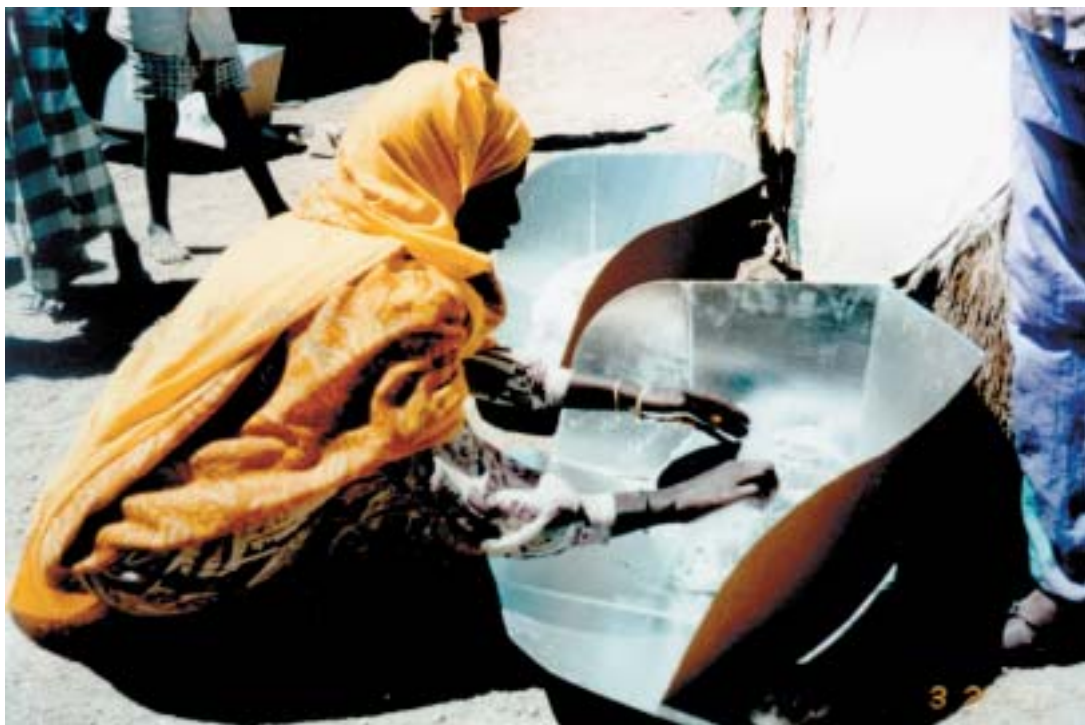
A foldable solar cooking kit saves fuel in a Kenyan refugee camp.
