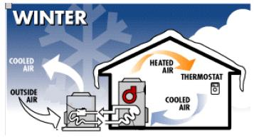
Air Source Heat Pump (ASHP) Principle: Air, at any temperature above absolute zero contains some heat. An ASHP transfers some of this heat from one place to another – for example between the outside and inside of a building. This can provide space heating and/or hot water.
