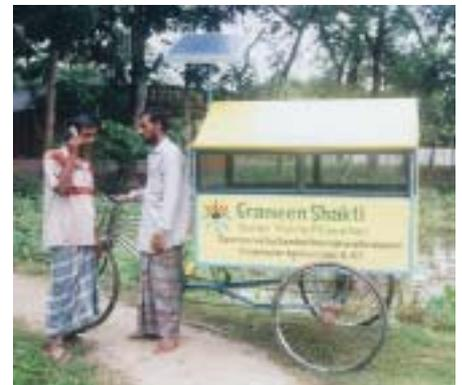
One new use of SHS is for mobile phone charging devices. At present, almost every corner of Bangladesh is covered by mobile phone signals, but many people cannot utilize this technology due to lack of mobile phone charging capabilities. GS has developed mobile phone charge sets. Every month about 500 mobile phone charging sets are sold with the SHS.
