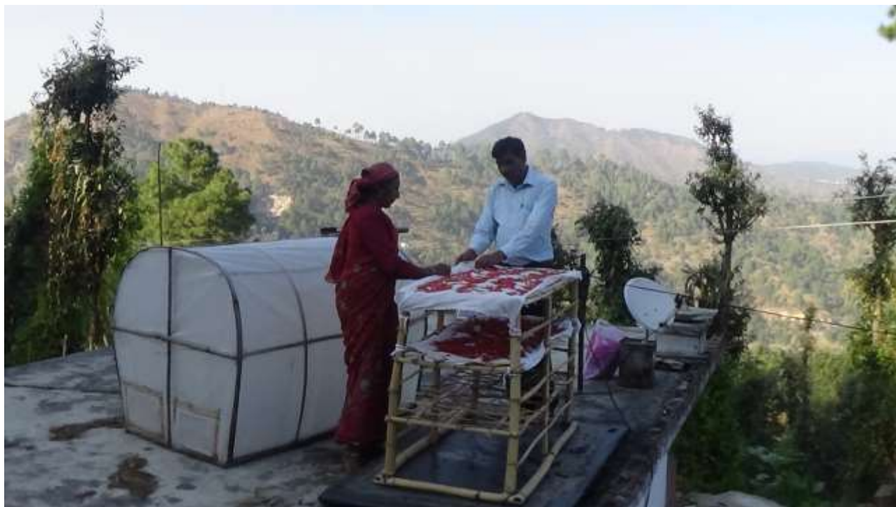
Photo: Solar tunnel dryer for small farms and households. The photo shows vegetables being loaded on the dryer's trays. Photo by INSEDA, India
