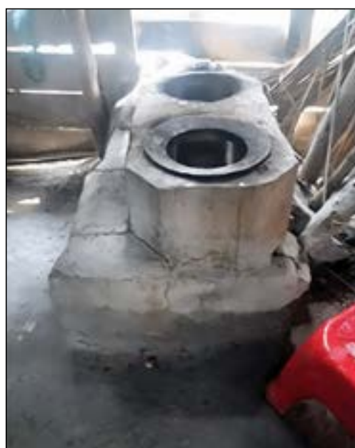
Durable concrete 2-pot improved cookstove. Photo by Grameen Shakti
