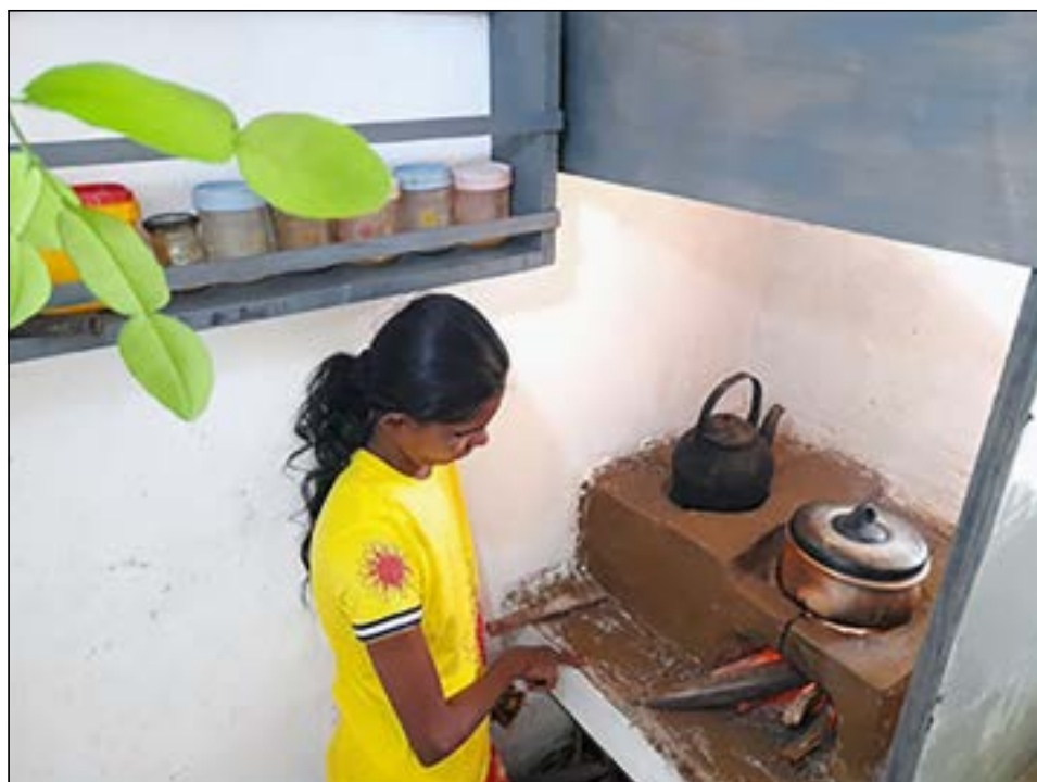
Improved biomass 2-pot cookstove and best practice with chimney hood. Photo by IDEA
