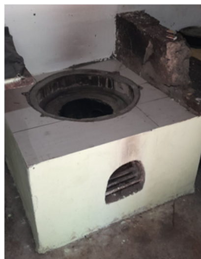
Top: Kottawatte Village in Southern Sri Lanka. Left: Household cookstove (Anagi) installed in the village. photo: IDEA. Right: Industrial stove installed in the village, photo: IDEA
