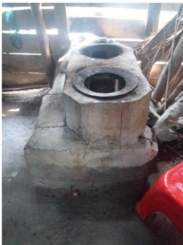
Left: Two-pot improved cookstove in Majherchar, Bangladesh model. Right: Biogas plant in Majherchar Village, photos by INFORSE
