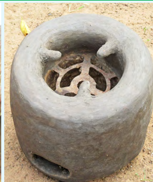
Innovation - modified shielded firewood stove by Yellow Power Women's group in Nebbi subcounty
